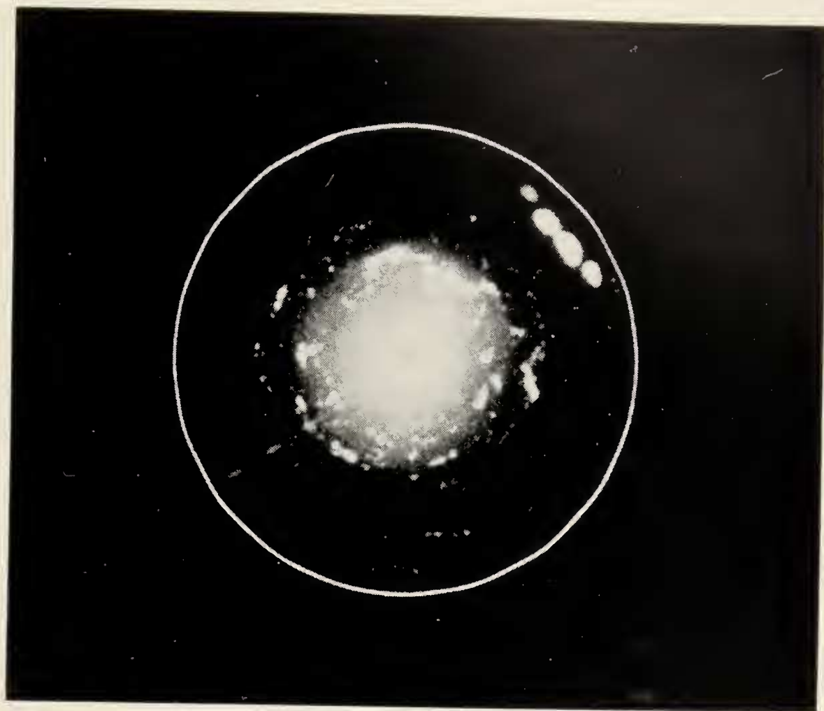
FIG. 6. Enlargement of 16-mm-radar-film frame (2-minute exposure) showing presentation on radar indicator with antenna on 30^\circ (above horizontal) scan. Large white spots near range mark show track of airplane intercepted in four rotations of the radar beam.
